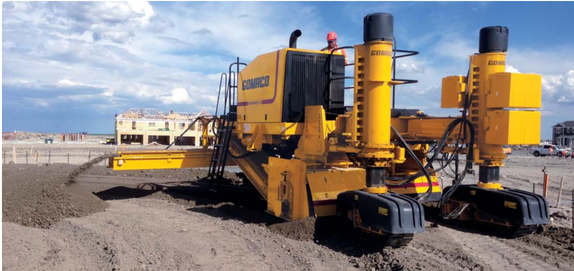
The Commander III trimmer is equipped with a powerful trimmerhead with 114 horsepower (85 kW) of the total power of the engine dedicated to it.
