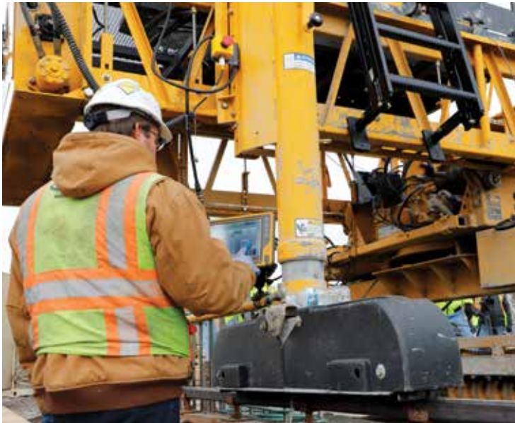
The C-450 and high-production screed can be controlled by a touchscreen on ground level. With the operator being at ground level, they can view exactly what the machine and high-production screed is producing so they can control how far to advance it or what changes need made during the paving process.
